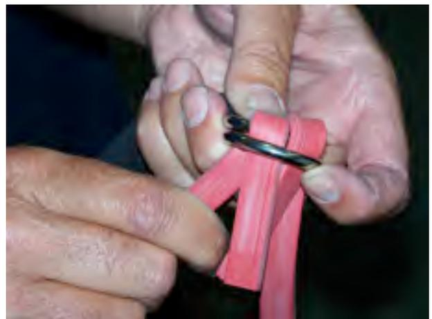
Push D-rings together – tighten down band
